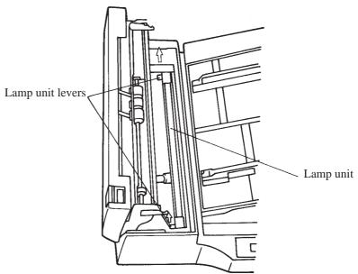
Figure 5.5 Lamp unit removal 2
